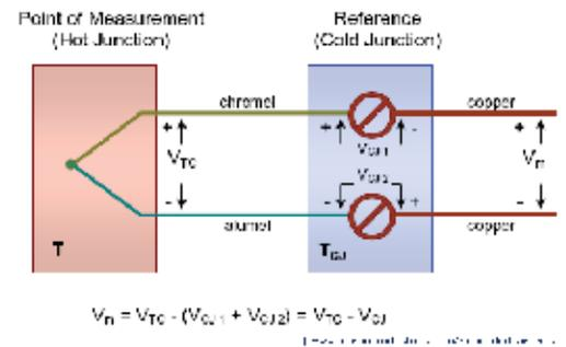
Electronics International instruments provide a temperature compensating diode located right at the terminating end of the TC wire. This insures accurate temperature measurements.
