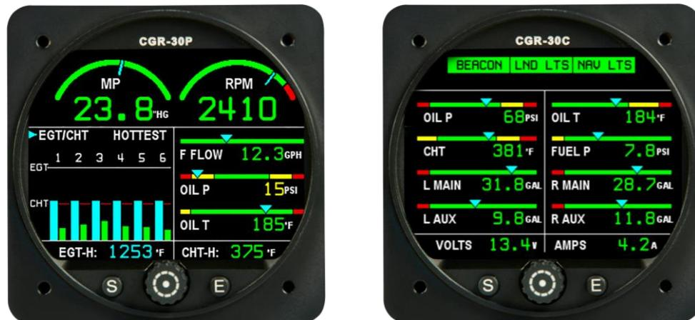
The CGR-30P and CGR-30C systems are identical in hardware, installation and maintenance. The difference between the two models is the configuration of the user screens. The CGR-30P incorporates two arcs at the top of the display, a bargraph display for monitoring EGTs & CHTs and strip gages for other functions. The CGR-30C only displays strip gages.
