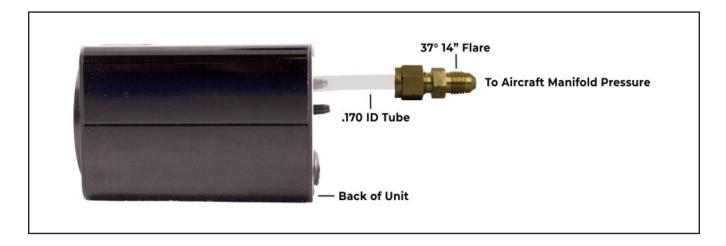
**Note:** Some aircraft have a very small hole in the manifold pressure line to create an airflow in the line. This small flow of air keeps fuel from working its way into the manifold pressure gauge or tranducer whitch can cause damage over time.
