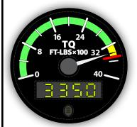
Electronics International Inc. will configure the TR-1-TQ to the range limits provided by the pilot/owner and/or mechanic. The data provided must match your aircraft's POH/AFM and all changes required by AD's, Supplements and/or STC's. Also, limits may be crosschecked against the instrument previously mounted in the aircraft panel. If any of the information provided on this form is incorrect and requires a reconfiguration, there will be an additional fee.
