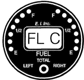
8. Toggling the Selector Switch from the center position to the left or right will change the resolution ("GAL1" or "GAL.5").
