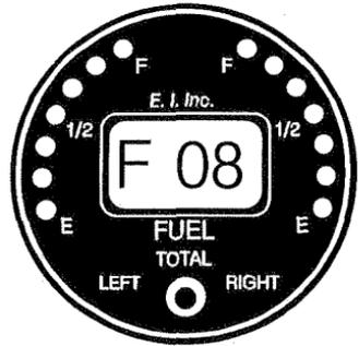
5. Once you have selected the filter setting, tap the Enter Button on the back of the FL-2 to display the current operating mode. The programmable letters will be blinking.
