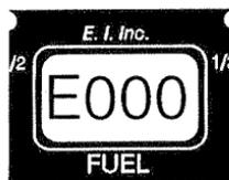
To program (change) the fuel level for this calibration point, push and hold the Enter Button on the back of the FL-2 for 3 seconds. To change the blinking digit, move the Selector Switch from the center position to the left or right. To blink the next digit to the right, tap the Enter Button on the back of the FL-2. To exit the programming of the fuel level for this calibration point and stop the blinking of a digit, push and hold the Enter Button on the back of the FL-2 for 3 seconds.
