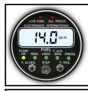
Electronics International Inc. will configure the FP-5L to the range limits based on the data provided by the pilot/owner and/or mechanic. The data must match your aircraft's POH/AFM and all changes required by AD's, Supplements and/or STC's. Also, limits may be cross-checked against the fuel pressure instrument previously mounted in the aircraft panel. If any of the information provided on this form is wrong, there will be a fee to change the configuration.
