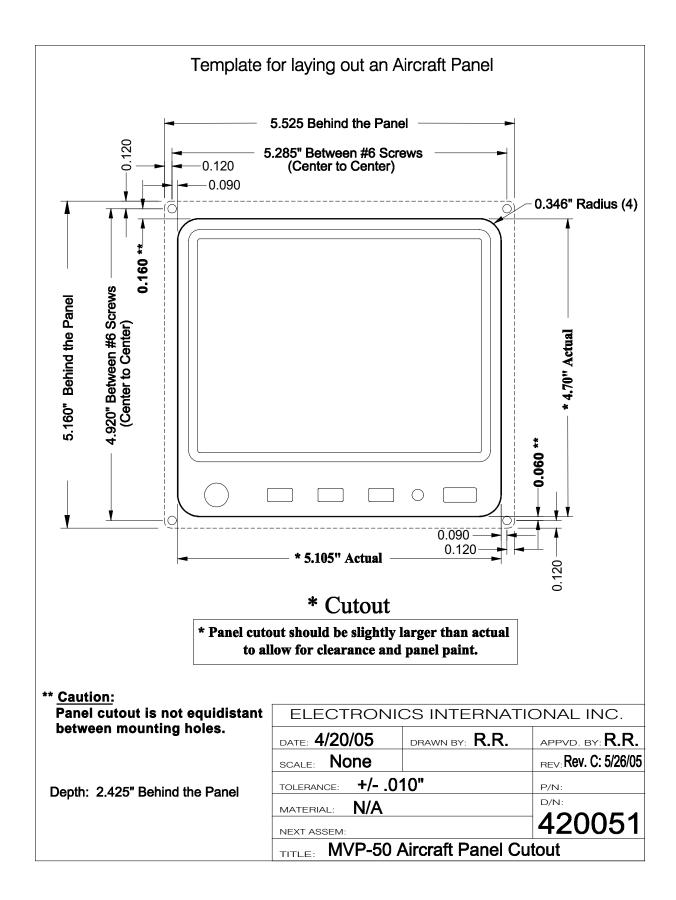
Note: A MVP Sub-panel can make installation of the MVP display much easer. See the E.I. Price List for more infromation.
