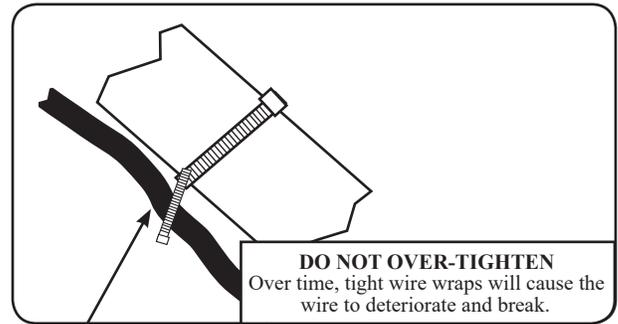
Use two zip ties when securing the probe to the airframe, this will help prevent probe failure due to excessive vibrations. One zip tie to attach to the airframe and one to attach to the cable. The wire should not touch metal, nor should any zip tie be so tight as to cause pinch points to occur.
