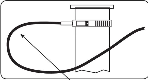
Provide a service loop for the probe cable. This will allow for engine movement and vibration.
