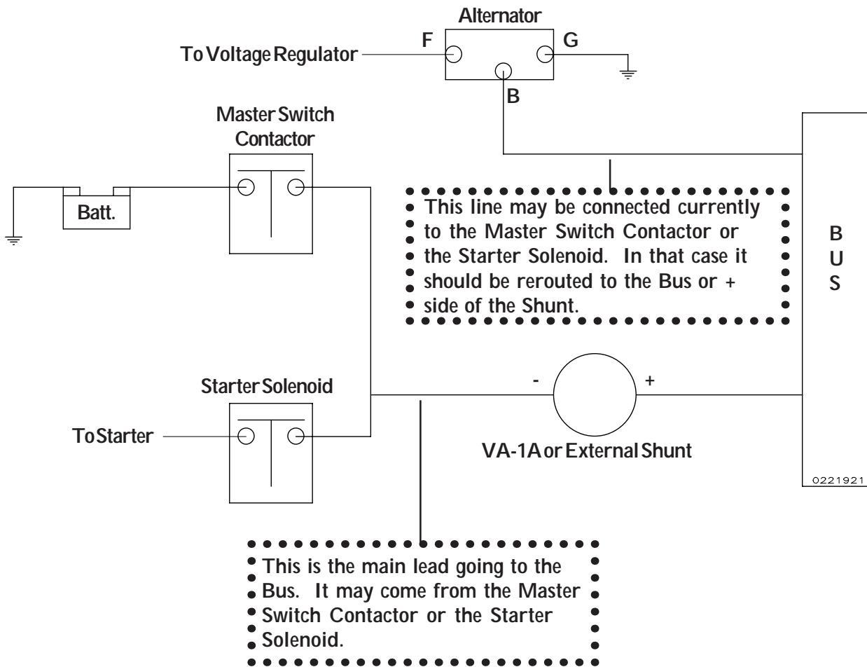
Note: The VA-1A or External Shunt should not be installed in series with the starting current.
