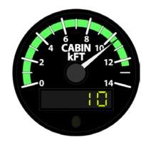
Electronics International Inc. will configure the TR-1-CP to the range limits based on the data provided by the pilot/owner and/or mechanic. The data must match the aircraft's POH/AFM and all changes required by AD's, Supplements and/or STC's. Also, limits may be crosschecked against the instrument previously mounted in the aircraft panel. If any of the information provided on this form is wrong, there will be a fee to change the configuration.
